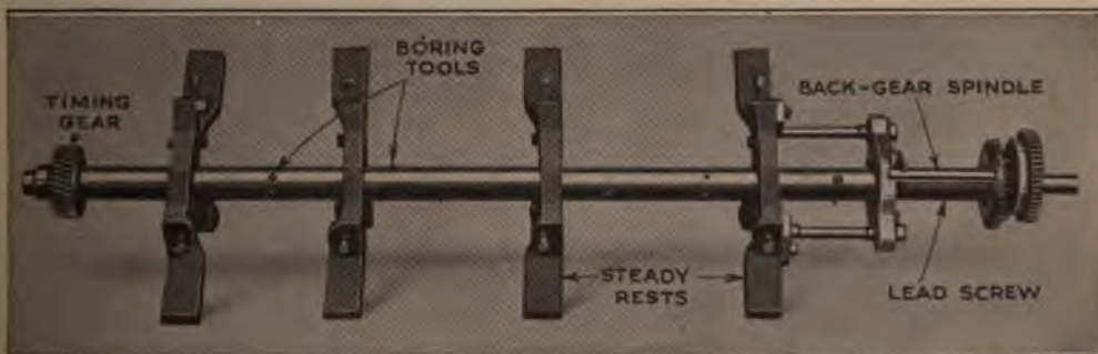
The Bar, the Steady Rests, and the Feed Mechanism in Position: The Spindle of the Back Gears is Extended, and is Held from Turning by a Dog, Attached to the Built-Up Nut. Four Steady Rests are Used in Working on the Six-Cylinder Engine
